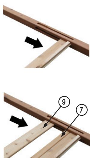
Install one 31" x 2-1/2" narrow center side rail (Item 7) and slide down. Install one 31" x 5-1/2" side rail (Item 9) and slide down.
