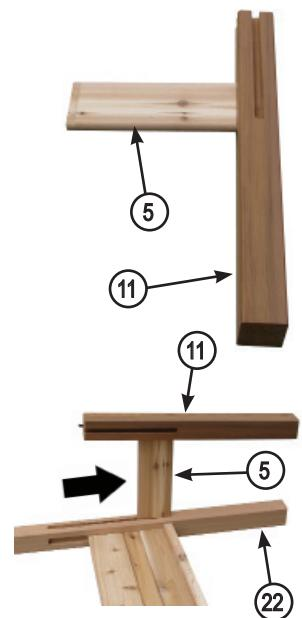
Rotate the 4" x 4" x 32" corner post (Item 11) and the 14-1/2" x 5-1/2" side rail (Item 5) 90°, install the side rail into the upper (wide) part of the slot on the 4" x 4" x 80" corner post (Item 22) and slide down to the bottom of the slot.
