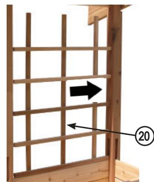
Align the the top of the trellis on the center of the top side rail, center the trellis left and right and fasten with six 8 x 1-1/2" screws (Item 14) on top & bottom of trellis.
