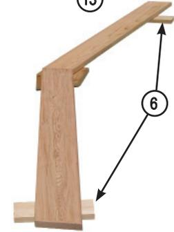
Place a support plate (Item 12) onto the top of the two trusses. Align the support plate with the top and bottom of each truss. Verify that the two trusses are still contacting each other under the support plate.
