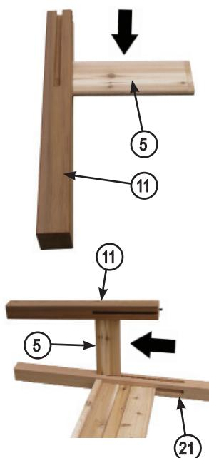
Rotate the 4" x 4" x 32" corner post (Item 11) and the 14-1/2" x 5-1/2" side rail (Item 5) 90°, install the side rail into the upper (wide) part of the slot on the 4" x 4" x 80" corner post (Item 21) and slide to the bottom of the slot.
