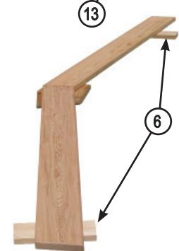
Place a support plate (Item 12) onto the top of the two trusses. Align the support plate with the top and bottom of each truss. Verify that the two trusses are still contacting each other under the support plate.
