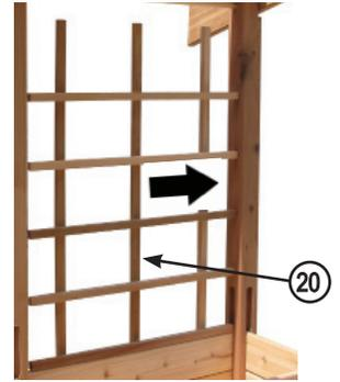
Align the top of the trellis on the center of the top side rail, center the trellis left and right and fasten with six 8 x 1-1/2" screws (Item 14) on top & bottom of trellis.
