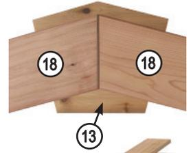
Adjust the trusses until centered left / right and up / down on the pentagon cap. Place one bottom board (Item 6) under each truss. This will help level the trusses.
